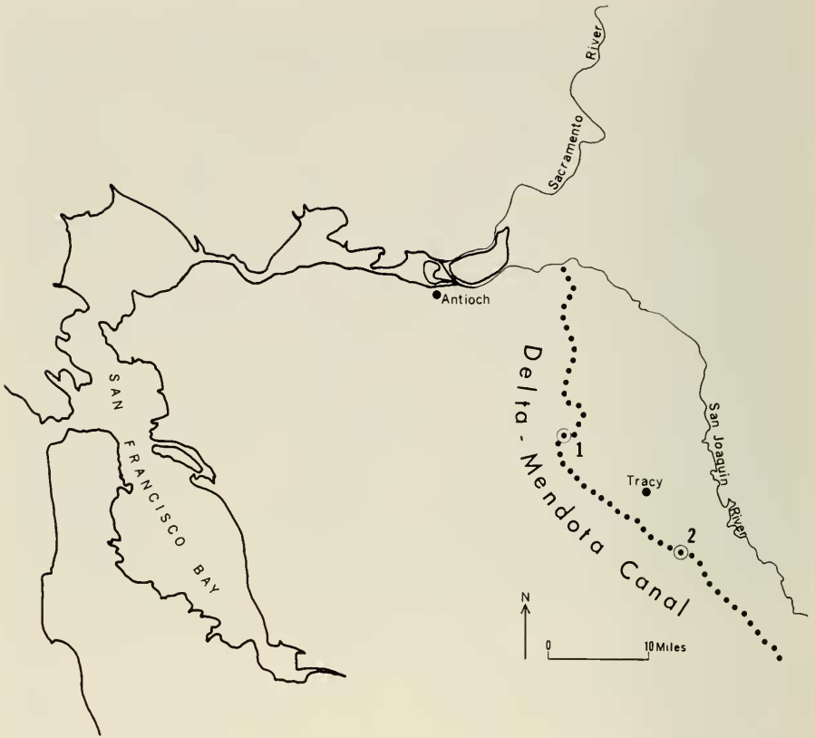
FIGURE 7. Relationship of Delta-Mendota Canal system to the San Francisco Bay-Delta area. Numbers indicate Tracy Pumping Plant (1) and collection site of Balanus improvisus (2).
